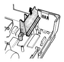
7. Remove the shield plate above the parallel interface by pressing in on the plastic clips located at the back of the plate. (The following illustrations show a rear view of the printer.)
